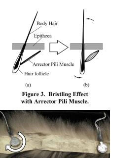
Figure 4. Disk-shaped Vibration Motor To Provide Horizontal Vibration.
